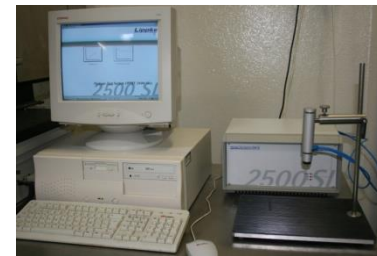
Leak and seal strength test
